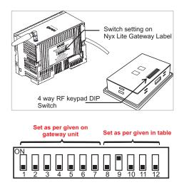
b) The remaining 5 DIP switches (Switch 8 to 12) are meant for room location of the device. Choose the location and set the DIP switch setting as shown in below table:
