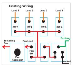
4. Identify Raw Phase, Inverter Phase and Neutral wire from switch board and connect it to respective terminal of RF Compact Four Switch Module. 5. Remove load wire Load 1, Load 2, Load 3 and Load 4 from switch board and connect them to Nyx Switch module on location marked as L1, L2, L3 and L4 respectively.
