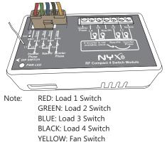
8. If user wants to control all loads with inverter phase or Raw phase. Short raw phase and inverter phase terminals with the help of short link and connect inverter phase or raw phase.
