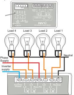
9. Like light loads user can connect and control fan regulator (NDMR1010) with RF compact Four Switch Module. For fan regulator wiring refer fan regulator manual.
