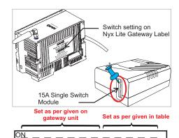
b) The remaining 5 DIP switches (Switch 8 to 12) are meant for room location of the device. Choose the location and set the DIP switch setting as shown in below table:
