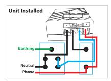
10. Fit RF Single 15A Switch Module by adjusting wires and insert module inside wall cavity, screw the switch board.
