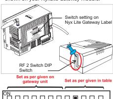
b) The remaining 5 DIP switches (Switch 8 to 12) are meant for room location of the device. Choose the location and set the DIP switch setting as shown in below table:
